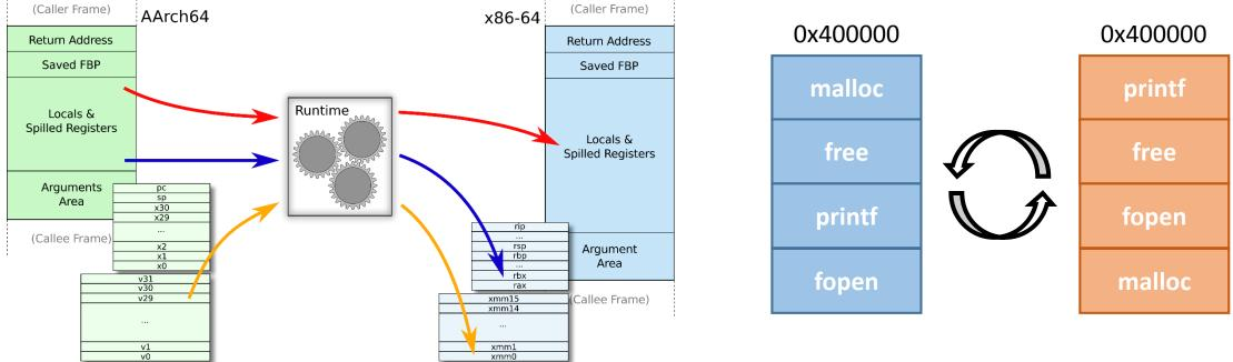
Inter-ISA migration limits the ability of attackers to chain together gadgets and gives a limited lifetime to the usefulness of any leaked memory layout information
