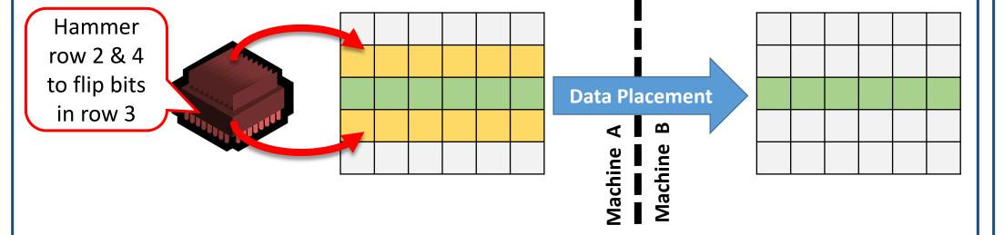
• Secure Popcorn allows transparently placing critical data in physically isolated memory, nullifying traditional information leakage/side-channel attacks
